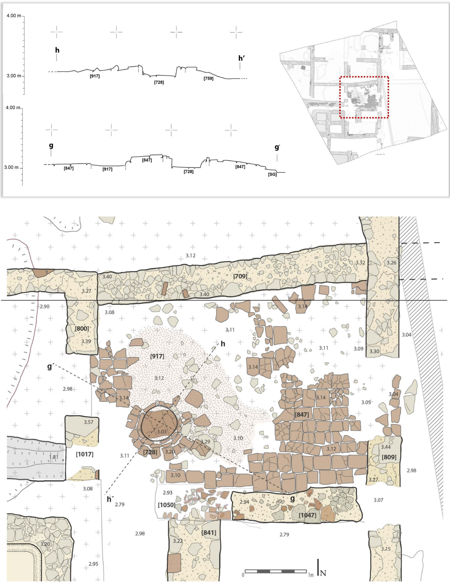
Figure 2. Final plan and sections of space VI in the fish-salting complex, including the glass furnace.
