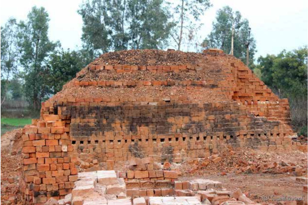
Image 7: Pajawa or Clamp Kiln. Photograph Suyash Dwivedi, https://en.wikipedia.org/wiki/Kiln#/media/File:Indian_brick_kiln.jpg
