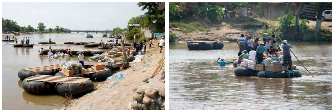
Figure 1 A crossing along the Suchiate River near the border cities of Ciudad Hidalgo in Mexico, and Tecún Umán, Guatemala. The rafts that cross the Suchiate River are made of wood planks lashed to inner tubes of tractor tires
